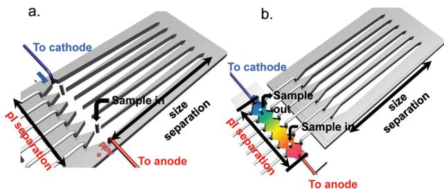
**Figure 1.** Schematics of IEF-AF4 channels with (a) an IEF segment embedded in a multilane AF4 channel and with (b) a separate IEF channel connected to a multilane AF4 channel. The connection between each electrode and IEF segment was made with Teflon tubing filled with electrolyte solution, leading to each electrolyte reservoir.
