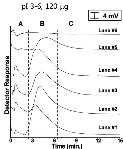
**Figure 3.** IEF-AF4 separation of human urinary proteome using ampholyte solutions with pH = 3.0–6.0 under the same experimental conditions used in Figure 2. Protein fractions were collected for shotgun proteomic analysis at the end of each channel during the time interval marked in broken lines.
