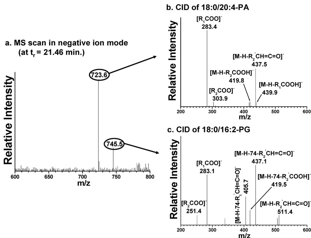
**Fig. 4** (a) Precursor MS scan at a retention time of 21.46 min (Fig. 1b) in negative ion mode. MS/MS spectra of (b)  $m/z$  723.6 (identified as 18:0/20:4-PA) and of (c)  $m/z$  745.5 (identified as 18:0/16:2-PG).
