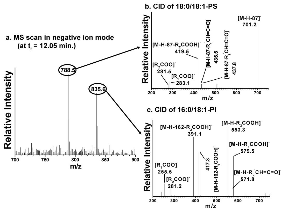
**Fig. 3** (a) Precursor MS scan at a retention time of 12.05 min (Fig. 1b) in negative ion mode. MS/MS spectra of (b)  $m/z$  788.5 (identified as 18:0/18:1-PS) and of (c)  $m/z$  835.6 (identified as 16:0/18:1-PI).
