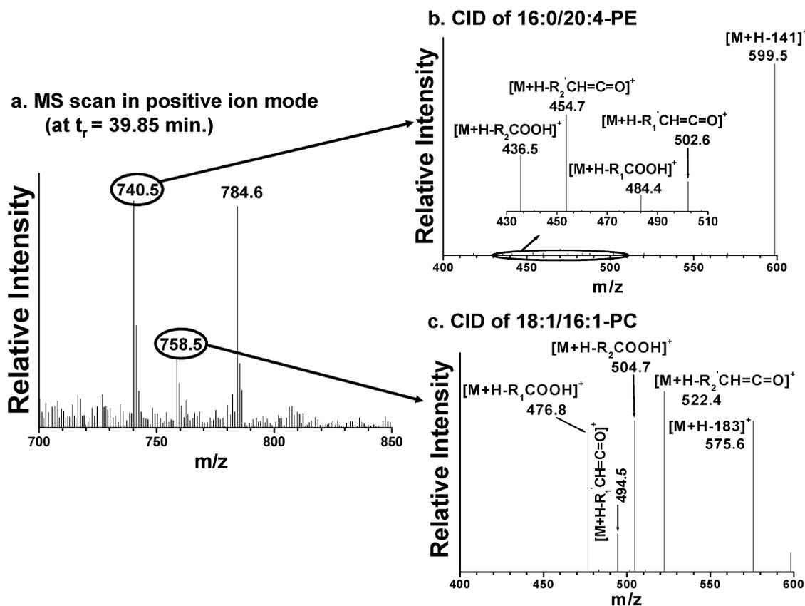
**Fig. 2** (a) Precursor MS scan at a retention time of 39.85 min (Fig. 1a) in positive ion mode. Data dependent MS/MS spectra of (b)  $m/z$  740.5 (identified as 16:0/20:4-PE) and of (c)  $m/z$  758.5 (identified as 18:1/16:1-PC).
