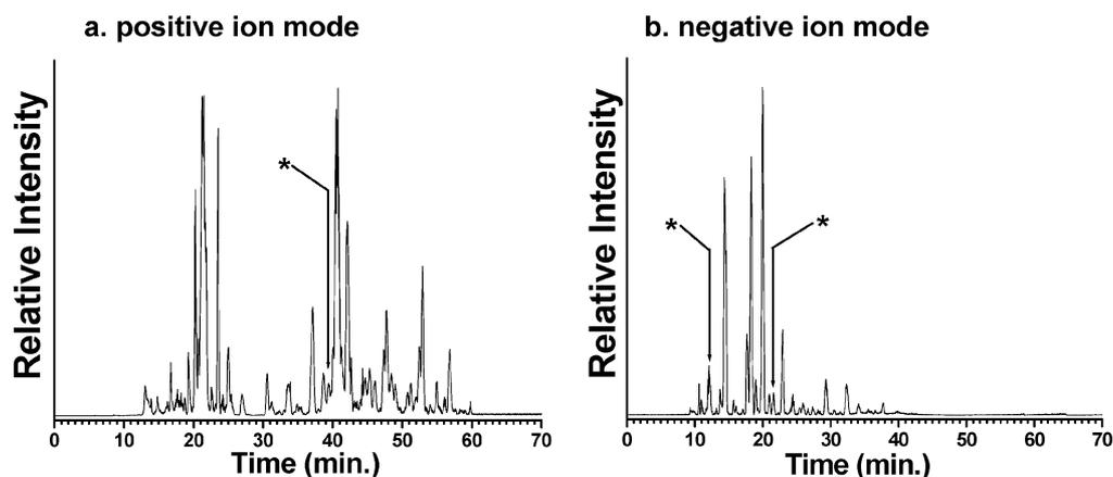
**Fig. 1** Base peak chromatograms of phospholipids extracted from 1 mL of human urine in (a) positive ion mode and (b) negative ion mode of nanoflow LC-ESI-MS-MS.
