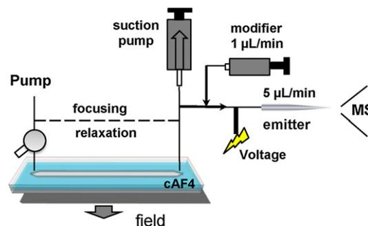
**Fig. 1.** Schematic of cAF4–ESI-MS-MS. The cAF4 effluent was split into two parts (4:1) with the aid of a syringe pump in suction mode, and the resulting flow directed toward the ESI emitter was premixed with ionization modifier liquid from another syringe pump.
