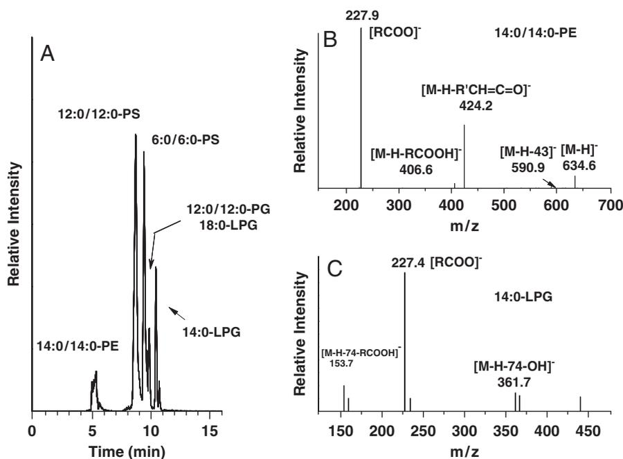
**Figure 4.** (A) BPC of OT-CEC-ESI-MS of six phospholipids at the negative ion mode; data-dependent MS-MS spectra of (B) 14:0/14:0-PE and (C) 14:0-LPG representing the characteristic fragment ions. Experimental conditions in run (A) were the same as those described in Fig. 3.
