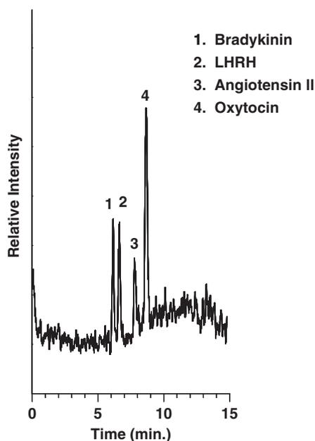
**Figure 2.** CZE-ESI-MS electropherogram of peptide standards (10  $\mu$ M each) obtained at 18 kV. For separation, an uncoated 50  $\mu$ m id  $\times$  30 cm fused-silica capillary column was used in 60:40 ACN/10 mM ammonium formate (pH 4) with a sheath flow (300 nL/min) of 50:50 methanol/water added with 0.2% formic acid.
