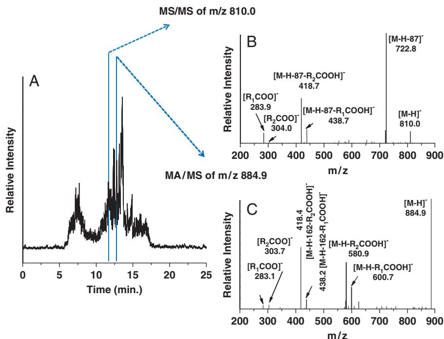
**Figure 5.** (A) BPC of urinary PL extracts from a healthy adult obtained by OT-CEC-ESI-MS at the negative ion mode along with MS-MS spectra of ions (B)  $m/z$  811.0 ( $t_r = 11.74$  min) and (B)  $m/z$  885.8 ( $t_r = 12.69$  min) during OT-CEC-ESI-MS-MS. Separation conditions were the same as those described in Fig. 3.
