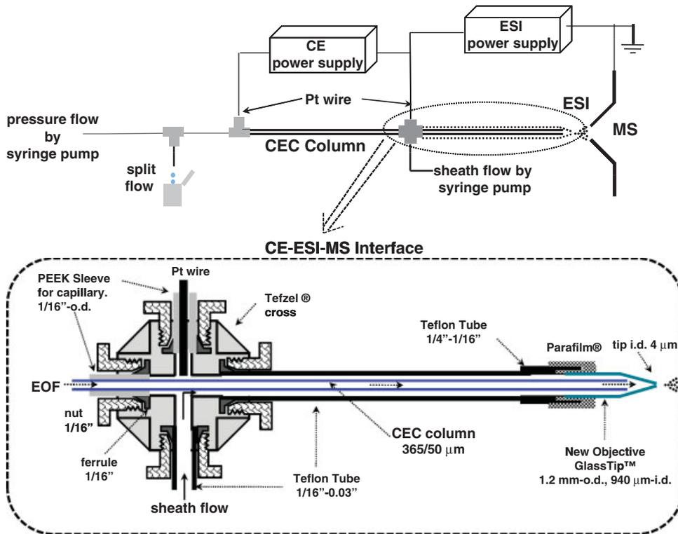
**Figure 1.** Schematic of the CE-ESI-MS; the interface developed herein is shown at the bottom.
