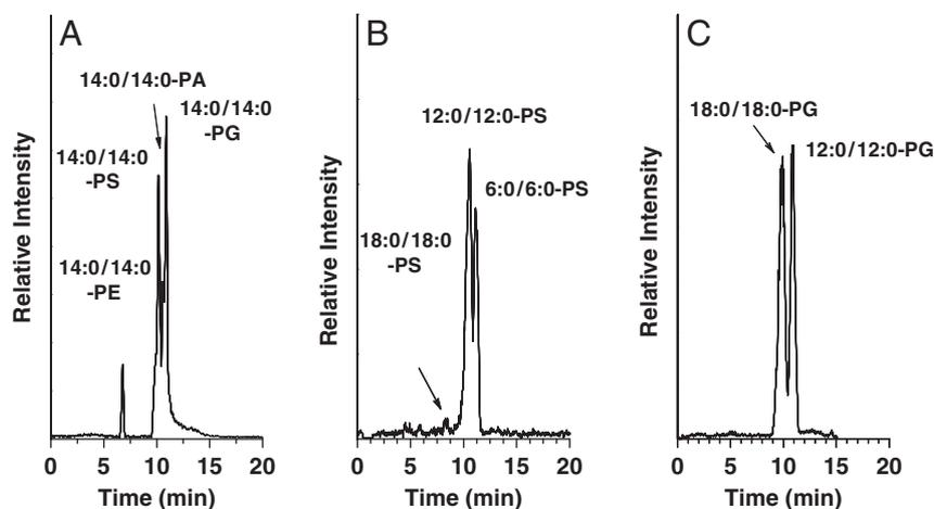
**Figure 3.** OT-CEC-ESI-MS electrochromatograms of (A) four PLs with different head groups having identical acyl chains (14:0 for both); (B) PSs; and (C) PGs with different chain lengths. An OT-CEC column with a polymeric monolithic layer was utilized in a solution of 60:30:10 isopropanol/ACN/50 mM ammonium acetate at 18 kV. ESI voltage at the negative ion mode was 2.2 kV with a sheath flow (500 nL/min) of 80:20 methanol/water added with 0.05% ammonium hydroxide.
