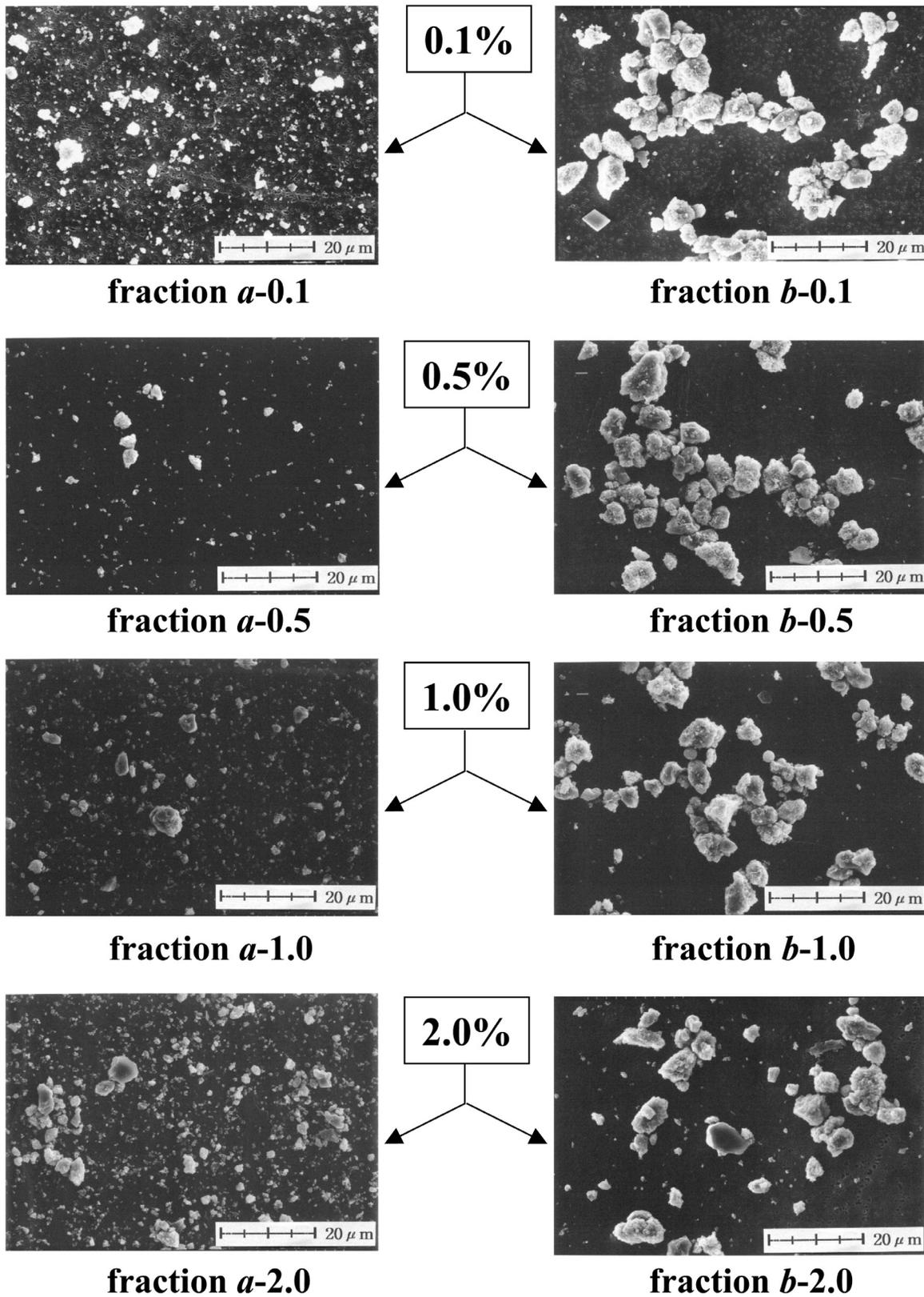
**Figure 5.** Electron micrographs of fractions collected at different feed concentrations using the pinched inlet GSF channel VI. Flow rate conditions are the same used in Figure 4.
