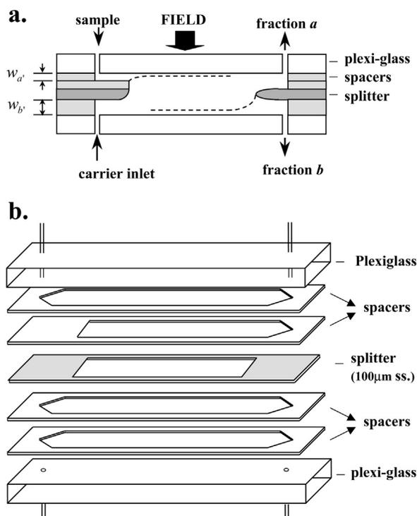
**Figure 2.** Schematics of the pinched inlet GSF channel: a) side view and b) the assembly of a pinched inlet channel.
