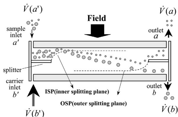
**Figure 1.** Schematic side view of SF channel.
