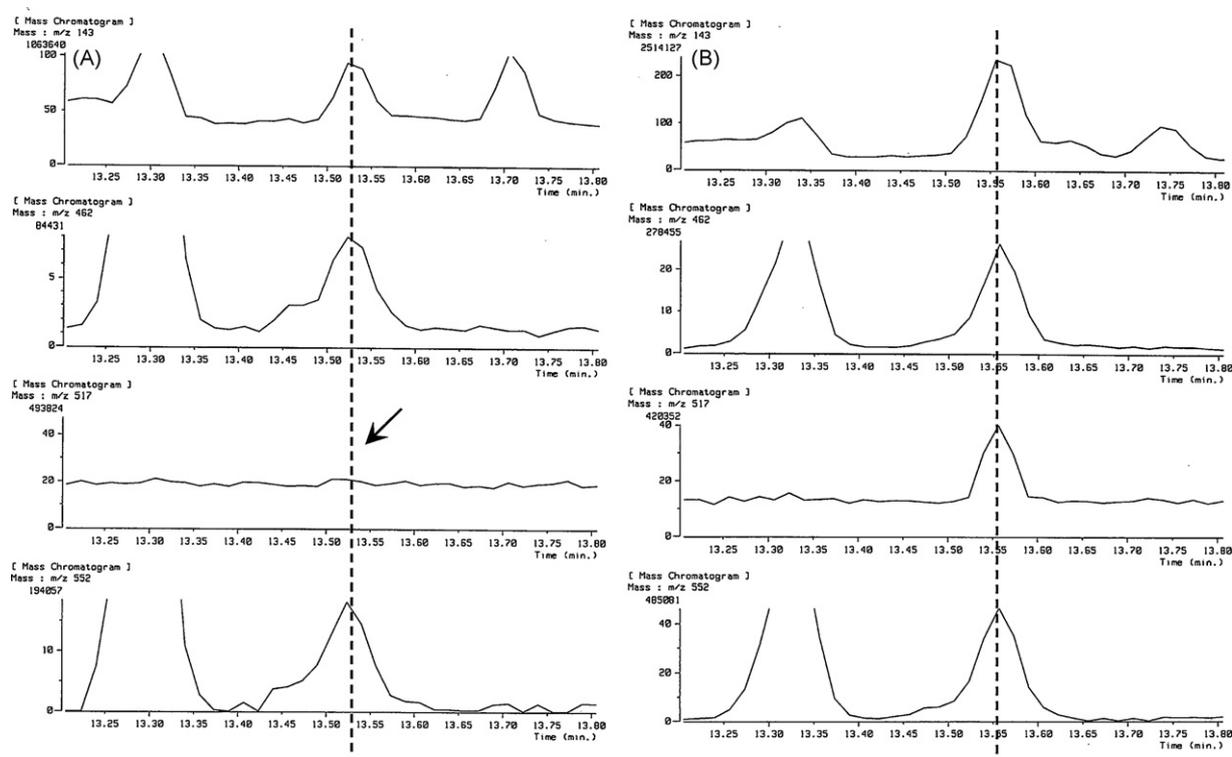
**Fig. 2** – Extracted ion chromatograms of fluoxymesterone-M1 purified with (A) Oasis HLB and (B) entrapped  $\beta$ CD polymer. The spectrum of fluoxymesterone-M1 as its tetra-TMS derivative has characteristic ions at  $m/z$  143 (D-ring cleavage), 462 ( $M^+ - 180$ ), 517 ( $M^+ - 90 - 35$ ), and 552 ( $M^+ - 90$ ). No peak at  $m/z$  517 was detected in sample purified with Oasis HLB, while chromatograms at four ions monitored were clearly detected in  $\beta$ CD experiment.
