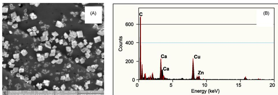
**Fig. 1** – Scanning electron microscope analysis of entrapped  $\beta$ -cyclodextrin ( $\beta$ CD) polymer. (A) The morphology at a magnification of 3000 of copolymer of  $\beta$ CD with epichlorohydrin treated with 0.3 M  $\text{CaCl}_2$  solution is presented. The entrapped  $\beta$ CD polymer by  $\text{CaCl}_2$  has relatively homogenous structure. (B) Compositional analysis shows presence of  $\text{Ca}^{2+}$  ions on the surface of polymerized  $\beta$ CD powder.
