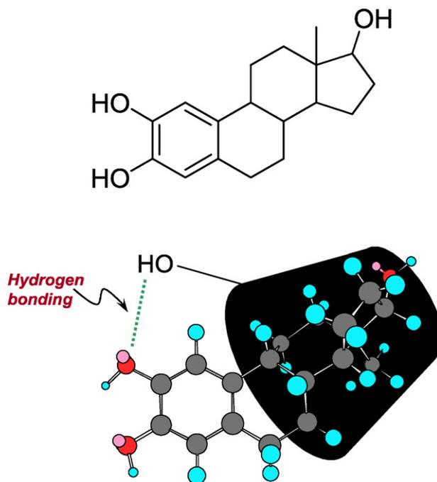
**Fig. 4 – Proposed inclusion complex of  $\beta$ CD with 2-hydroxyestrone. Some parts of the molecule are included into the cavity of  $\beta$ CD, and others are on the outside. The A-ring of steroid molecule is predominantly formed complexes with the  $\beta$ CD and its structural feature have a great influence on the stability of the inclusion complexes through the hydrogen bonding between phenolic hydroxyl and the exterior hydroxyl groups of estrogen and  $\beta$ CD, respectively.**
