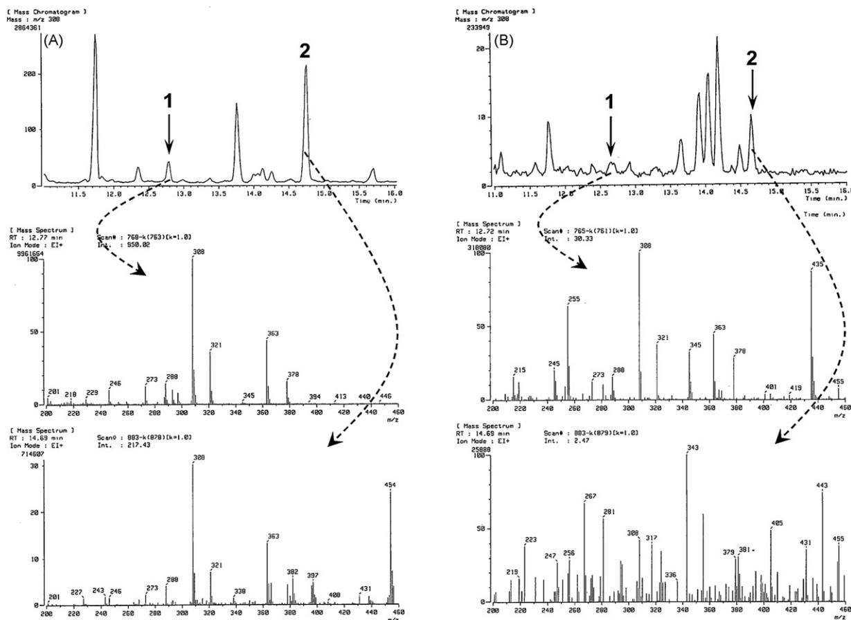
**Fig. 3 – GC–MS chromatograms and mass spectra for identification of oxandrolone and its metabolite epioxandrolone using (A) entrapped  $\beta$ CD polymer and (B) Oasis HLB. Total ion chromatogram shows selectively detected both (1) epioxandrolone and (2) oxandrolone. The characteristic ions ( $m/z$  308, 321, 363 and 378) for two compounds were clearly detected without any significant interference in the  $\beta$ CD experiment. The GC–MS conditions are listed in Supplemental Table 2.**
